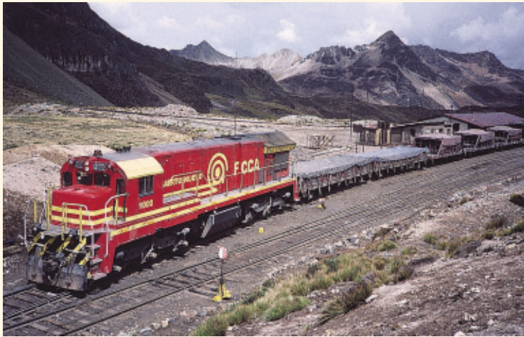
The five rebuilt GE C30-7 diesels offer increased haulage capacity and better fuel efficiency
