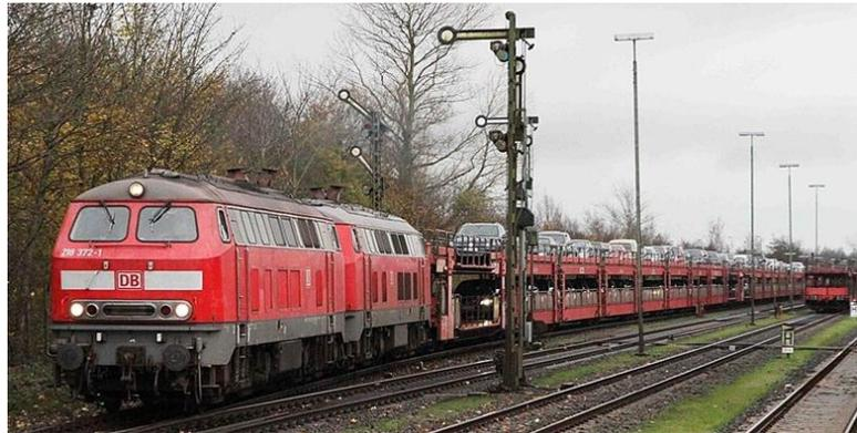
The existing Deutsche Bahn Sylt Shuttle uses diesel hydraulic locomotives built in the 1970s, although newer units are on order from Bombardier. A train is seen leaving Niebüll for Westerland on Nov. 18, 2014.
