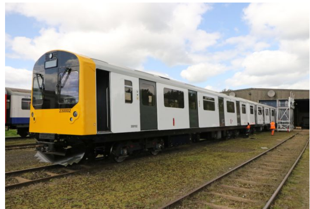
Prototype battery-powered class 230 unit 230 002 at Vivarail's base at Long Marston on May 10. Photo: Keith Fender
