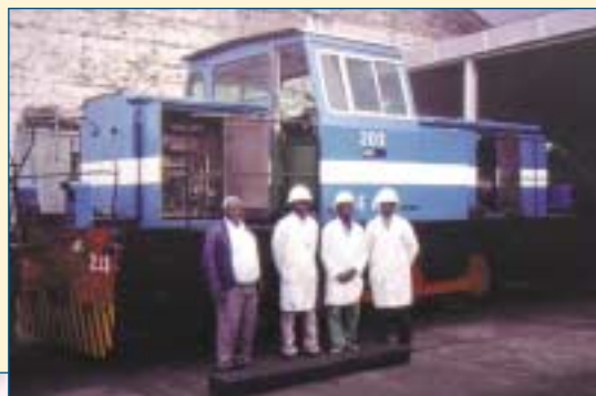
ABOVE: CEAR's Chief Mechanical Officer Bob Nkana (left) and the workshop team at Limbe overhauled this 1993-built CMI diesel shunter and modified the hydraulic drive to improve availability and reduce operating costs
