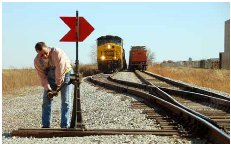
Conductor Stan Thomas lines a switch at Walcott, Iowa, to let his train, BICB, out on the main after a meet with its eastbound counterpart on Nov. 9, 2010. Fred W. Frailey
