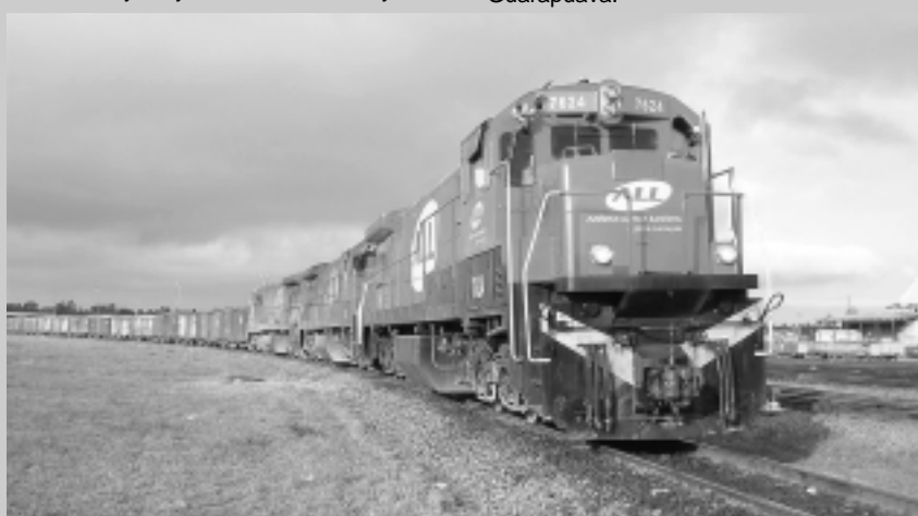
> Three GE C30-7s get ready to haul a long freight drag out of ALL's Punta Grossa yard. The standard gauge locos look enormous on meter gauge track.
