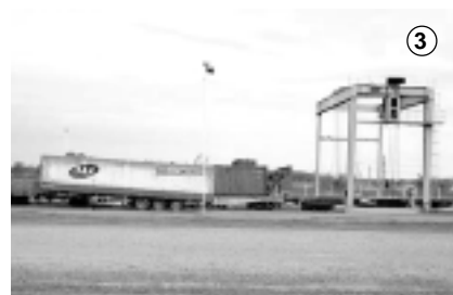
> (1-2) Westbound view of Zárate's intermodal terminal. The large shed, built at the yard's western end, facilitates cross docking and storage of paper products shipped by Alto Paraná, one of ALL Mesopotámica's major customers. (3) Zárate's intermodal terminal is equipped with a 50 ton rolling gantry. The 20-hectare facility was inaugurated in 2001. (J.C. González photo.)
