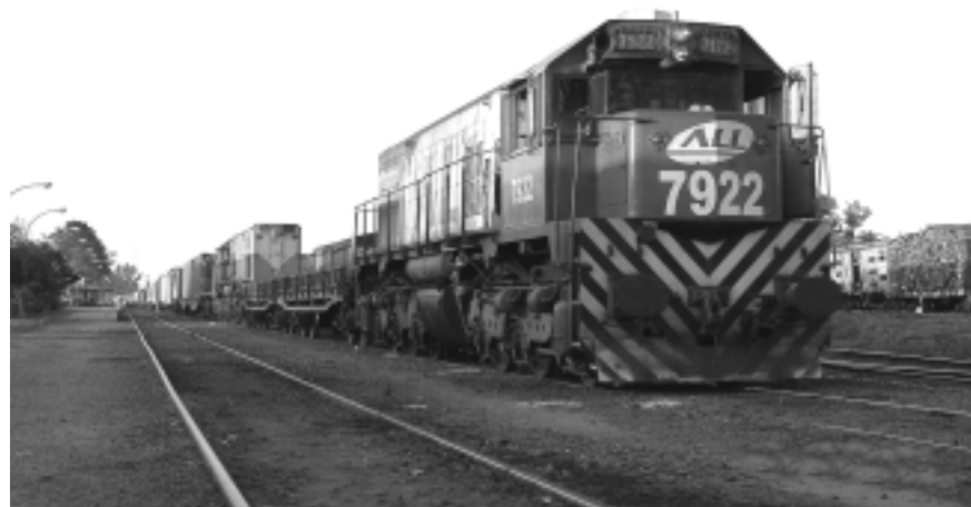
> Every day, at 06:00 PM, a 75 car train leaves Zárate headed northwards and 36 hours later (at 06:00 AM) it arrives at Paso de los Libres. The trains are usually double headed by two GMIC G22s separated by three low side freight cars, to spread the weight when traversing some of the old lightweight turn of the century iron pillared bridges. The two locos are capable of handling 4800 gross ton trains over ALL's Mesopotámica Division main line.
