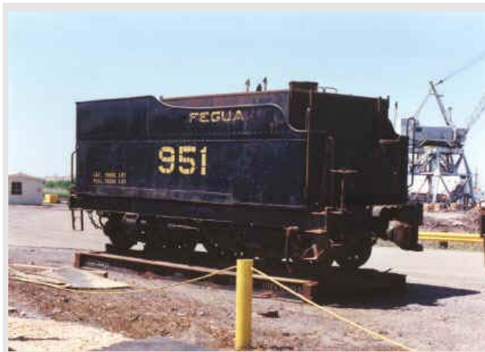
This tender was still in service in 1993 as a water car, and is the one working behind SVR #19 today. The oil tank had been boiled out, and was used for water storage, too.
