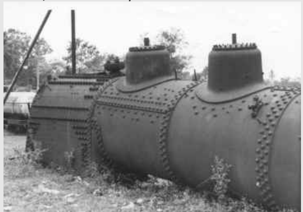
The second steam dome permitted an inspector to enter the boiler without removing the throttle valve.
