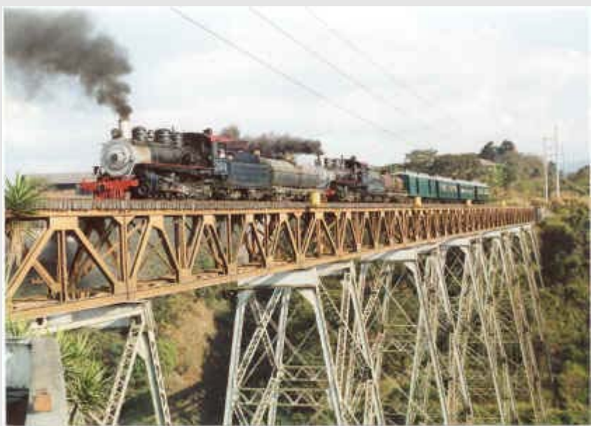
For many years, extra steam locomotive tenders were used to increase the operating range of engines in Guatemala. These days tank cars are preferred, as this view of #204 and #205 taken at Puente de las Vacas shows. Two of the most famous examples of FEGUA water cars were brought back to the USA and reunited with their original locomotives by the Sumpter Valley in 1993.
