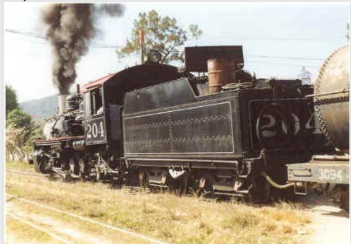
#204 heads for home. Level hose connection between tender and tank car feeds water without a pump.
