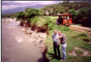
Another challenge is inspecting narrow gauge railways. In North America a Hy-Rail vehicle is used, meaning a highway vehicle with railroad wheels that drop down and operate on the track. You cannot use this method on narrow gauge because no one has built a pickup truck so narrow that it will work on the 3-foot gauge. Therefore track motorcars are used.
