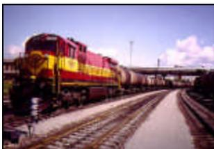
These are the used GE C36-7 locomotives that have been re-gauged and put into operation in Estonia. These off-the-shelf locomotives are replacing the Soviet locomotives on a 1-for-2 basis. I rode this particular locomotive when we set an all-time record for a single locomotive in Estonia – we hauled 5500 tons with one locomotive which had never been done before.
