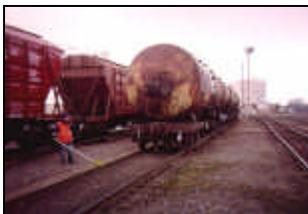
The other interesting thing for a North American is seeing wagons rolling through a yard and then noticing that there are no hand brakes. The Soviet legacy is a system, which is better than what we have in North America, of using skates. The man on the left is putting a metal wedge on the track called a skate; when the wagon hits the skate, it grinds to a stop. It is better than a hand brake because you cannot sabotage it or replace it by hand; you need a locomotive to pull it off.
