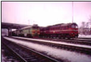
In the case of Estonia we inherited a Soviet locomotive fleet. These locomotives are maintenance intensive, fuel inefficient and highly polluting. We are in the process of replacing them with locomotives from North America.
