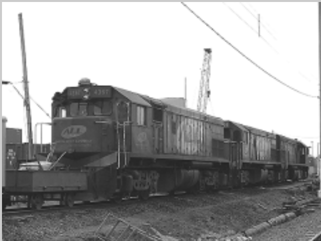
> Next to the station, parked on the loco pit stop's spur, there is a three unit lashup. The three locos are EMD G22s, which once refueled and serviced will be whisking a train out towards Sao Paulo.
